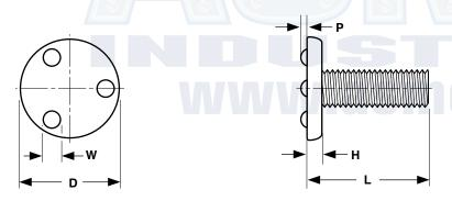
‡Length of a weld stud is measured from the welding surface of the head to the end of the shank, excluding the projections.
