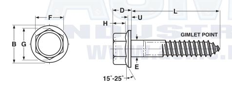
Length of a hex flange lag screw (L) is measured from the underhead bearing surface to the extreme end of the screw. Minimum thread length is 1/2 length of the screw plus 0.50 inch or 6 inches, whichever is shorter.
